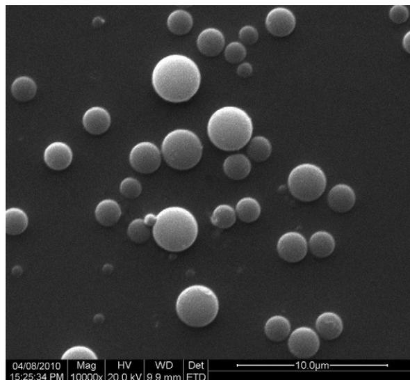
Fig. 2. Scanning electron microscope image of basic fibroblast growth factor 2–poly(lactide-co-glycolide) microspheres ( $\times 10,000$  magnification).
